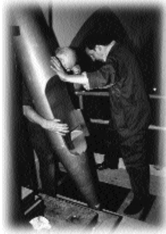
David Wood and Jim Beaver removing a pedal 16' Principal Pipe
